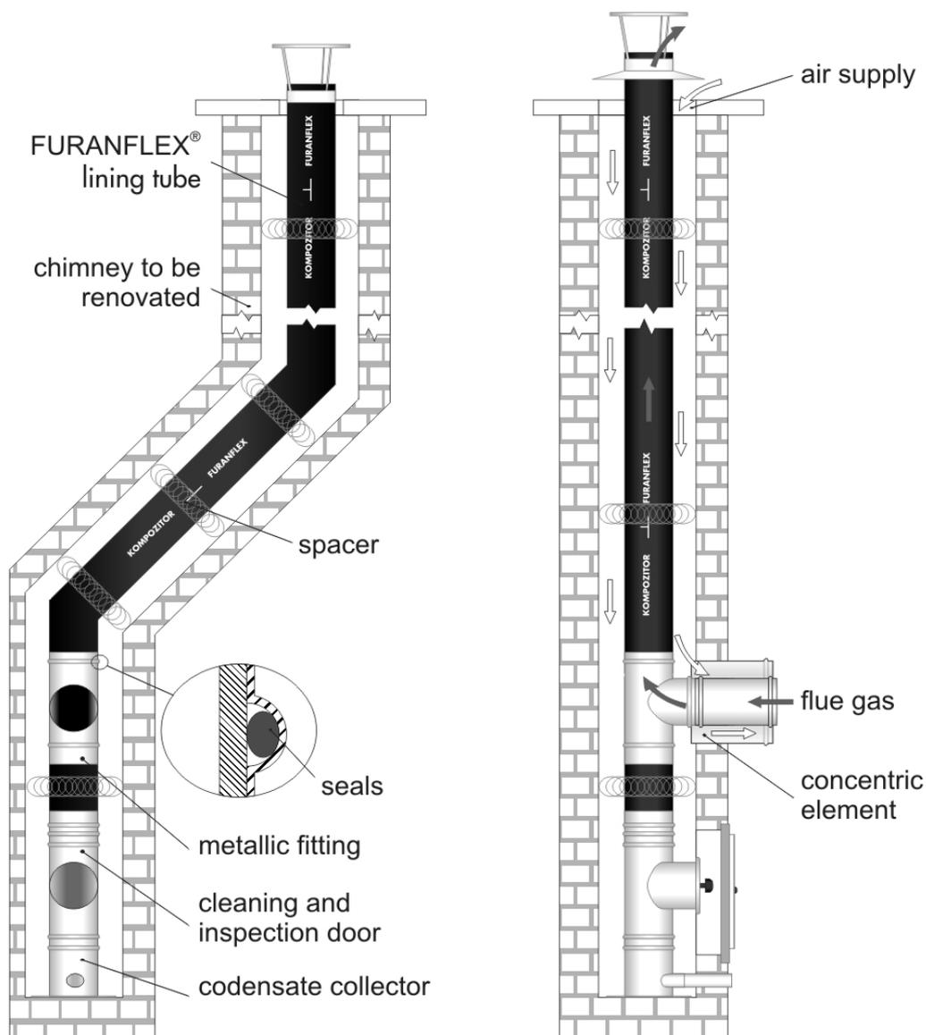
Figure left: Example for non-vertical installation (design situation no. 2)
