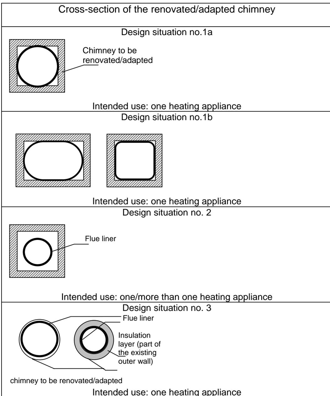
Note: Design situations given in 1a and 1b are representing similar situations for different cross sections of the chimney.
